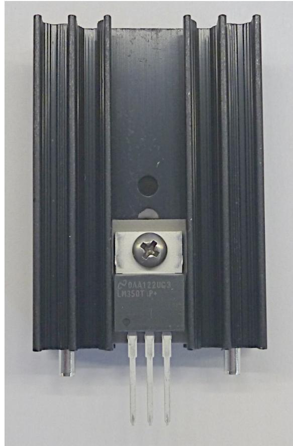
**Note one side of the heat-sink has narrowed fins, install the LM350 on THAT SIDE!**
