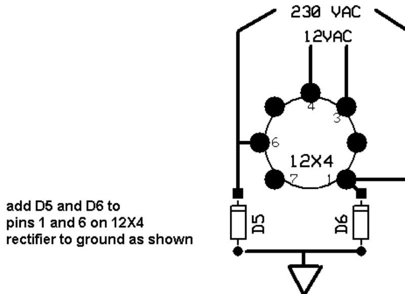
*The pin-out of the 12X4 above is shown looking from the TOP of the socket, NOT from the bottom!*
